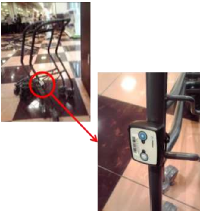
Fig. 1. An RFID tag is attached to each shopping cart.
